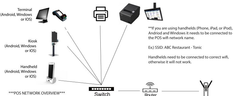
The restaurant needs to follow this diagram in order to have a well maintained POS network. Cabling needs to completed in order to connect all networking devices to the switch/internet. The following diagram gives an idea of what is recommended to complete the installation of your terminals. printers and networking
